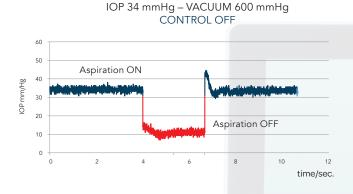
The chart shows IOP fluctuations under active aspiration without an IOP control system\*
